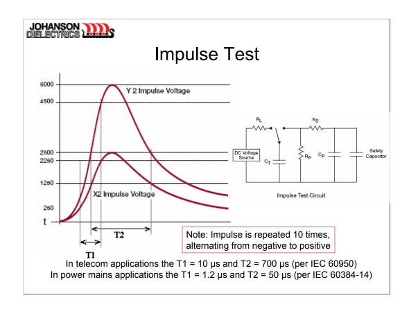
As mentioned in the previous slide, Safety Certified Capacitors are rated according to their impulse capability. Impulses are usually identified by their rise times (T1) and their time to half value (T2), and they are described as T1/T2 impulses (for example 1.2/50us impulse). The rise time is the time it takes the pulse to go from 10% to 90% of the peak voltage. T2 is the half value time and is the time it takes the voltage to go from 50% of the peak back to that same level.
