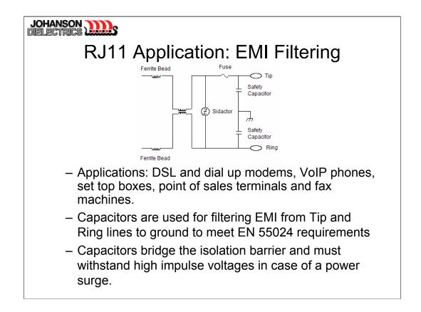
Safety Certified Capacitors are used in large quantities in telecom applications utilizing RJ11 (standard phone line) connections. These applications include DSL and dial up modems, set top boxes, VoIP phones, point of sales terminals and fax machines.
