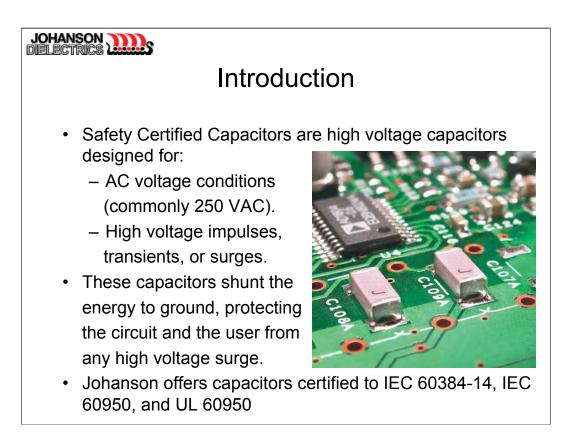
Safety Certified Capacitors are application specific high voltage capacitors that are designed to withstand AC voltage conditions and high voltage impulses. These capacitors shunt the energy from an impulse to ground, providing protection for the circuit as well as the end user. The capacitors offered by Johanson Dielectrics are rated 250VAC, and are certified to IEC 60384-14, IEC 60950, and UL 60950.
