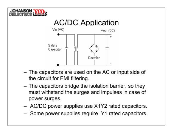
Another important application for Safety Certified Capacitors is in AC/DC power supplies. The capacitors are used on the AC or input side of the circuit for EMI filtering. Like phone lines, AC power lines carry a lot of noise as well as surges and transients. The capacitors bridge the isolation barrier, so they must withstand the surges and impulses in case of power surges.
