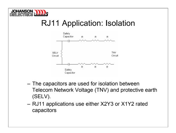
The second circuit where Safety Certified Capacitors are used is the isolation circuit. The capacitors are used for isolation between the Telecom Network Voltage (sometimes called TNV) and protective earth (sometimes called SELV). The values used in this circuit are usually less than 100pF.
