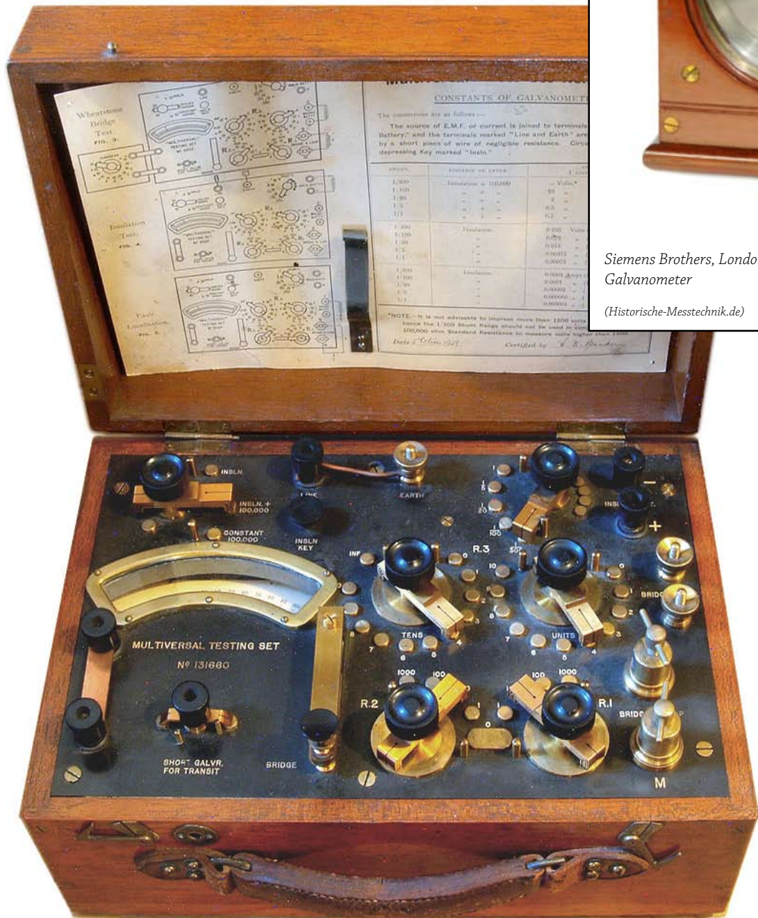
Siemens Brothers, London Universal-Galvanometer (Wheatstone-Brücke), 1924 (Flickr)
